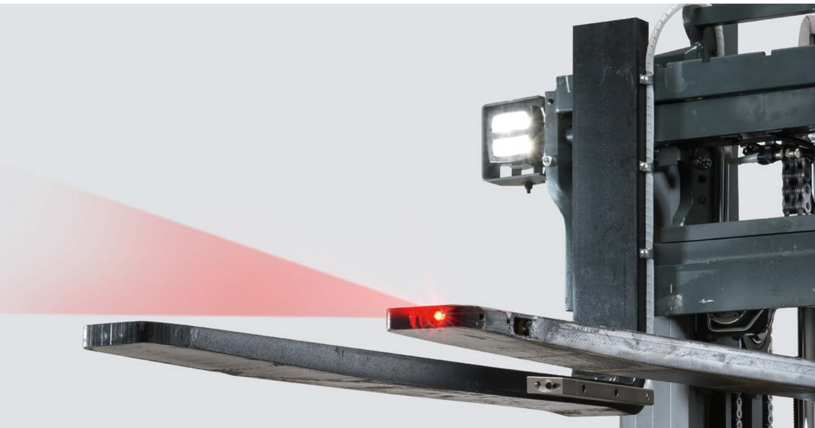
LED spotlights on the fork carriage with positioning laser
